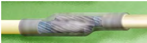
Figure 19-3. Sleeving over Soldered Connection
