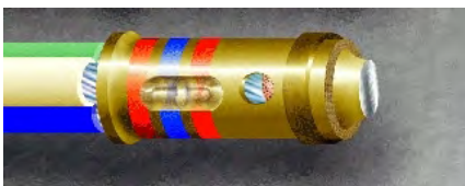
Figure 19-23. Contact Trimmed and Deburred
