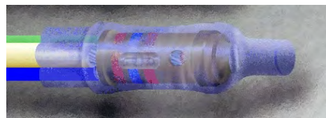
Figure 19-24. Contact Covered With Shrink Sleeving
