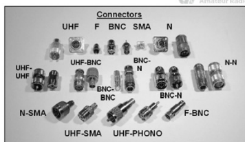
Figure 4.15 — The photo shows a variety of common coaxial connectors that hams use. The larger connectors are used for higher power transmitters and antennas. The most common are the UHF and N styles. Special adapters are used to make connections between cables and equipment that have different styles of connectors.
